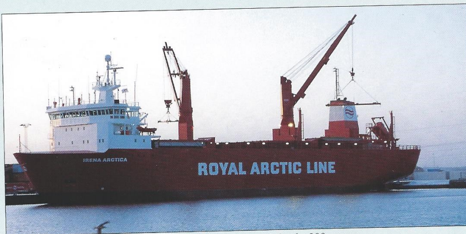
The forward location of the wheel house increases the visibility by 300 metres.
