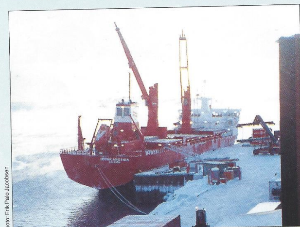
The Irena Arctica in the Port of Nuuk. Each of the ship's cranes can lift 40 tonnes.
